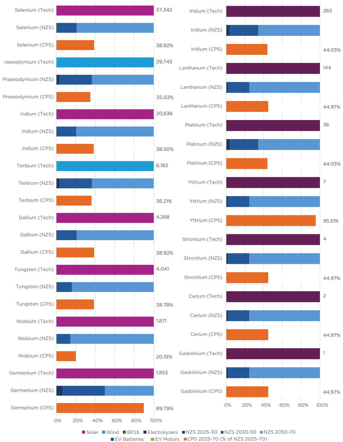
Figure 2.9b: Cumulative Mineral Demand in Current Policy Scenario (CPS) & Net Zero Scenario (NZS) (Interpretation of graph - Bar 1: Share across different technologies under NZS; Bar 2: Share across different time horizons under NZS; Bar 3: Proportion in CPS relative to the NZS; Secondary y-axis: - Total demand under the NZS (Tonnes) and percentage in CPS relative to NZS)
